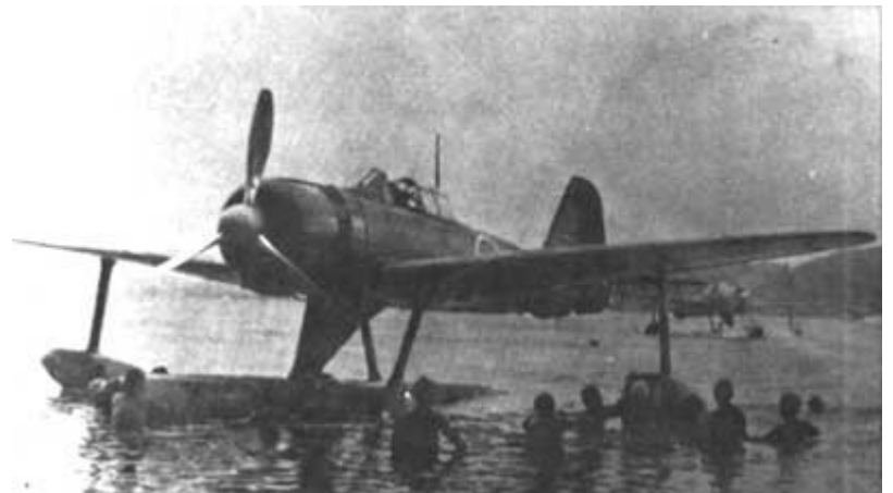
The A6M2-N float plane version of the Zero did extremely well, suffering only a small loss in its legendary maneuverability. Top speed was not affected, however, the aircraft's relatively light armament was a detriment.
